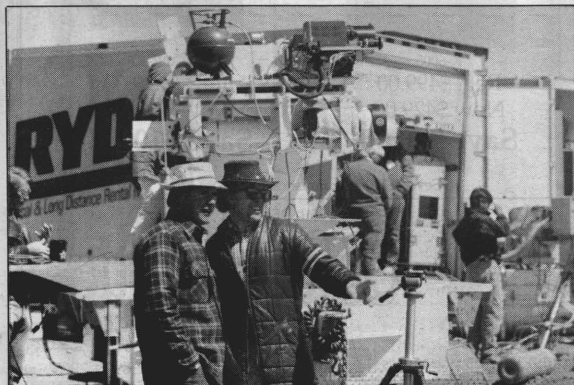
CATCH THOSE RAYS—A Mitsubishi 3-5M IR Imager tracks aircraft during Long Jump IV testing at White Mountain.
