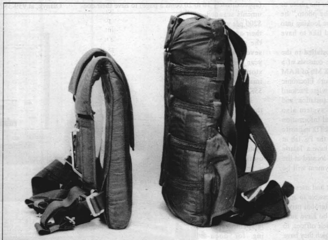
COMPARISON photo shows LESPA (left) as much smaller and cumbersome than the NB-8 it is being developed to replace. LESPA weighs just 17 pounds, compared to others at 25.
