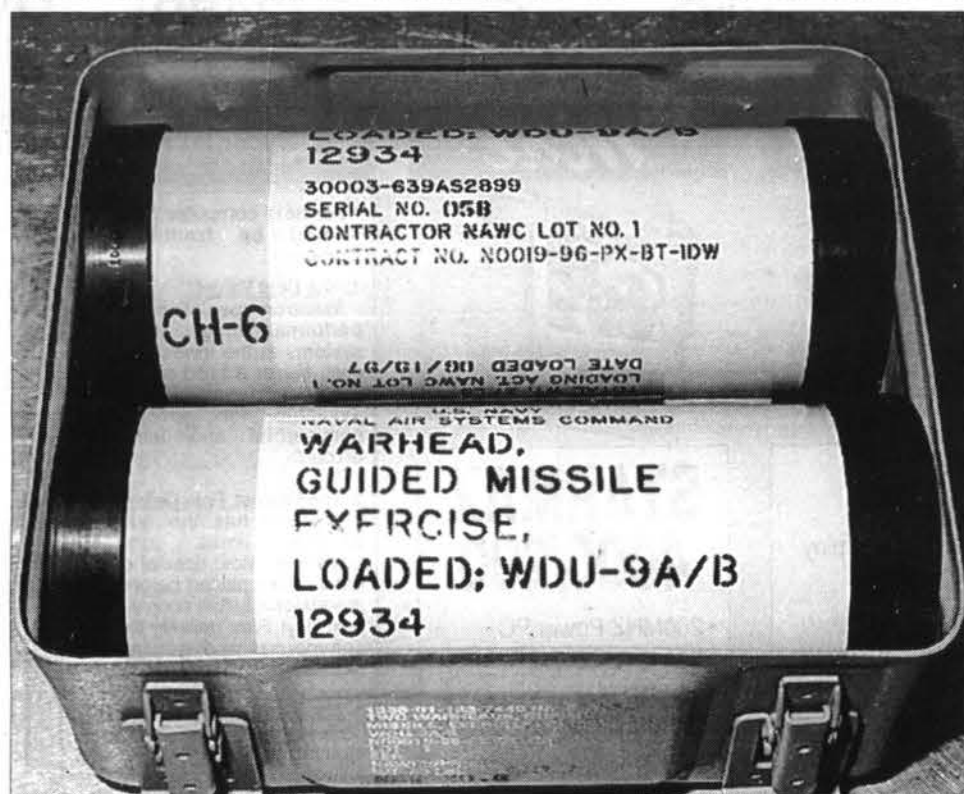
NONLETHAL —These Sidewinder Exercise Warheads (5x13"), packed for shipment to the fleet, will mark would-be kills while saving targets.
