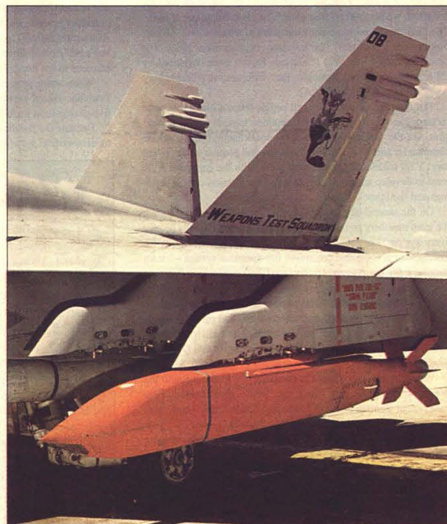
JSOW Unitary Test Vehicle (Variant 3) recently tested at NAWCWD includes improvements that will reduce costs during the production of all variants.
